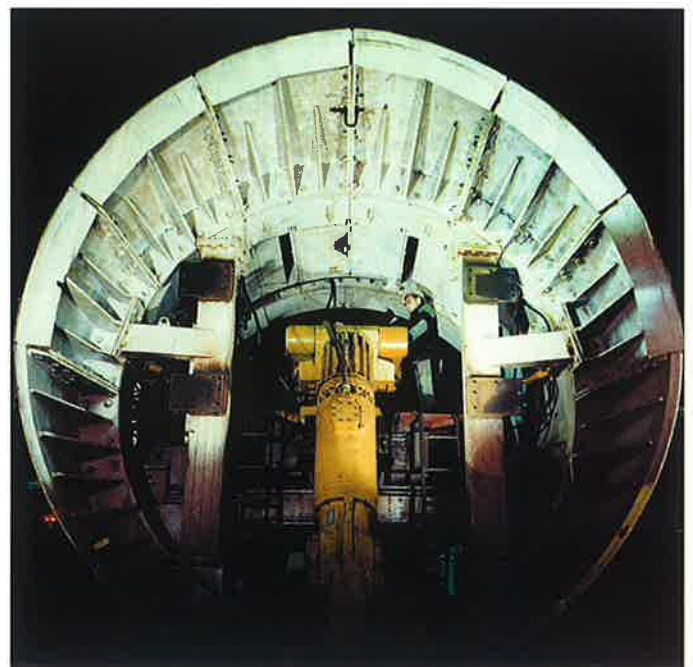
Obr. 4 Raziaci štít na razenie autotunela na magnezitovom ložisku Miková Fig. 4 Driving shield for the road tunnel driving at the Miková magnesite deposit
