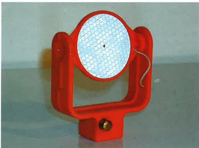
Obr. 2 Odrazné fólie v plastovém nosiči Fig. 2 Reflecting foils in a plastic holder
