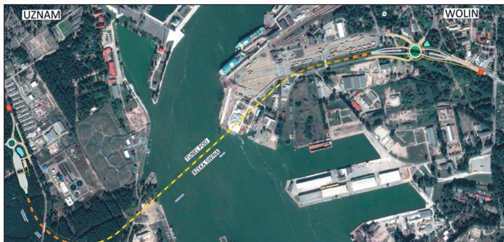
Obr. 1 Trasa 1,44 km dlhého tunela pod riekou Świna Fig. 1 Route of the 1.44km long tunnel under the Świna River
